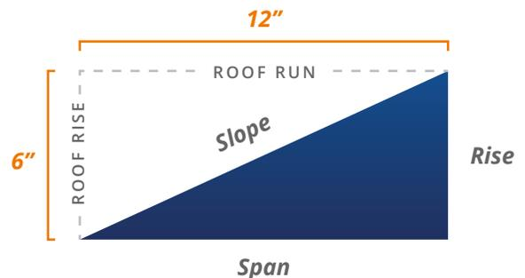
**ROOF PITCH = RISE / SPAN**
